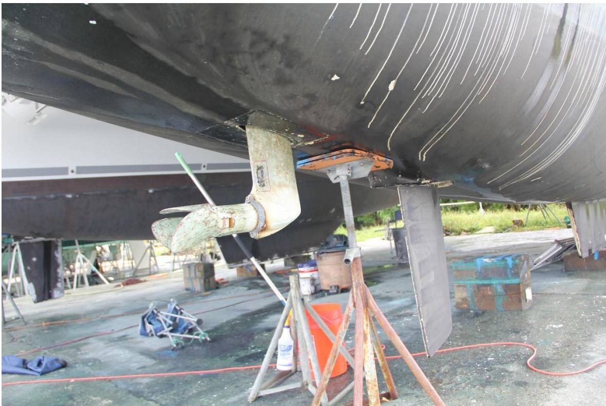
Starboard running gear, with SailDrive and folding propeller
