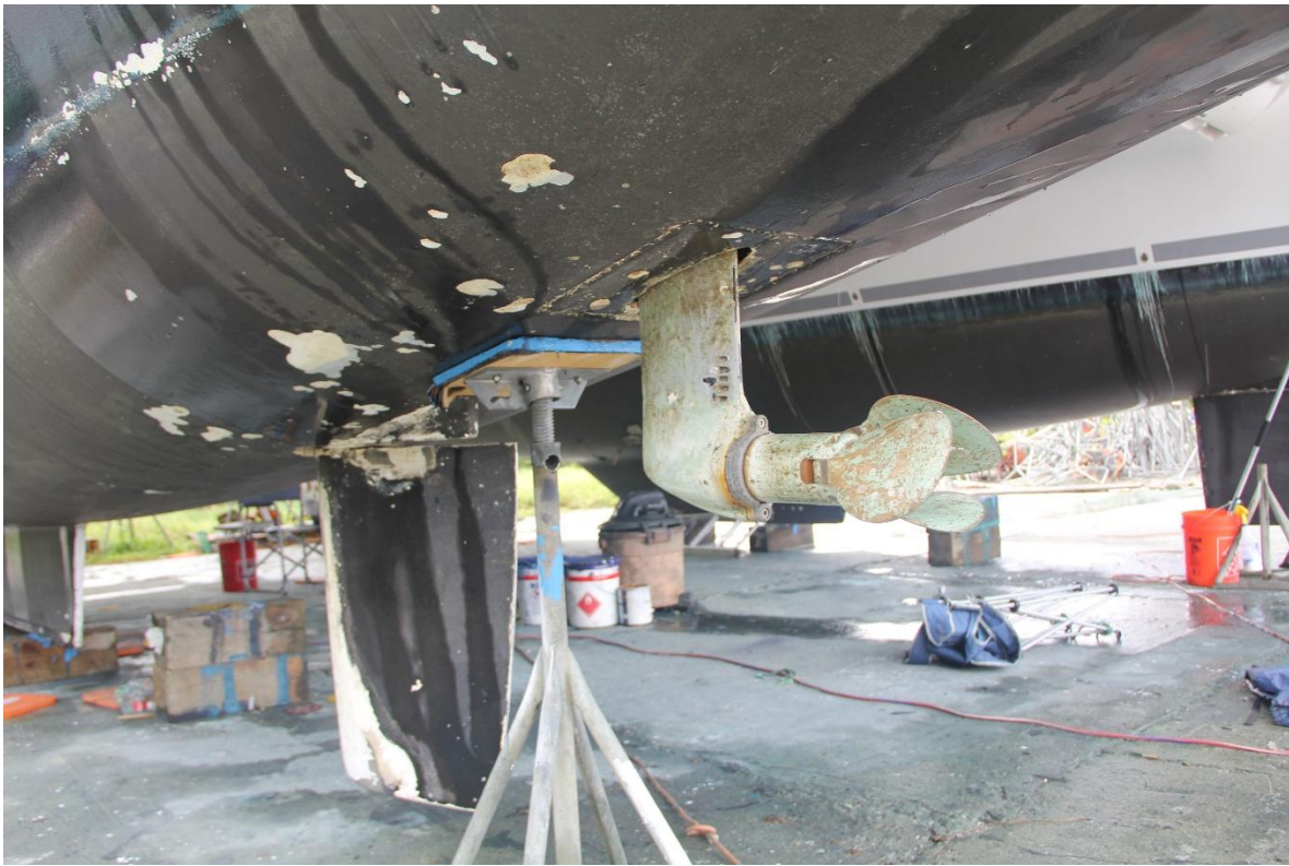
Port running gear, with SailDrive and folding propeller
