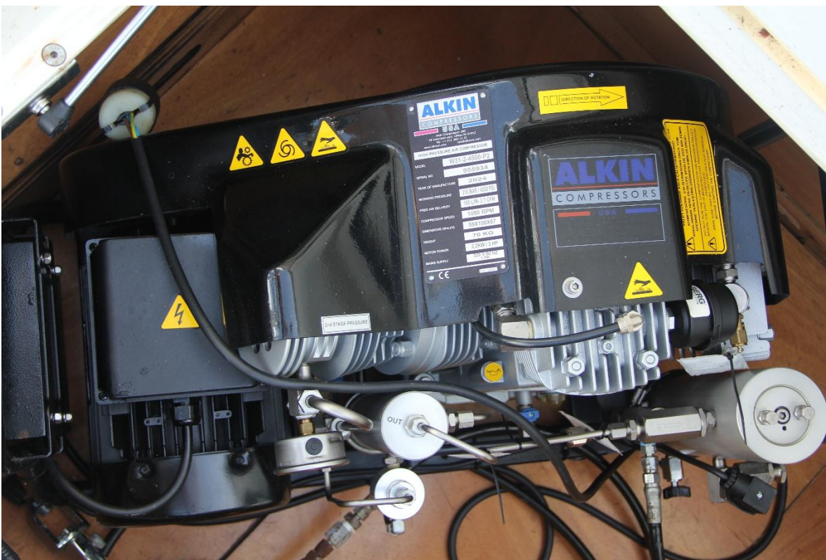
Alkin 3.7CFM 220V dive compressor; set above starboard engine/not removed
