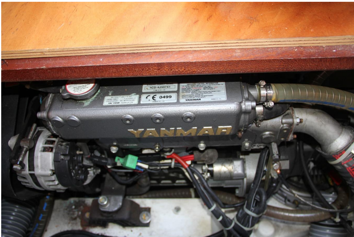
Starboard Yanmar 57HP diesel engine; where easily accessible
